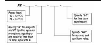
NOTE: Run output is 5 amp @ 12 or 24 VDC. Run output is the voltage required for an ignition system, fuel valve, or solenoid actuator that allows the engine to run.
